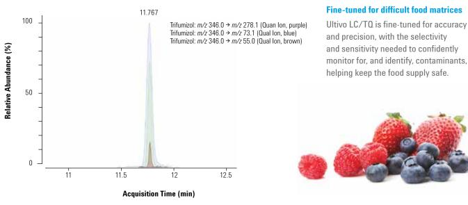
Quantitative analysis of pesticide residues in avocado matrix. Trifumizol is shown at 1.0 ng/g, demonstrating the excellent quantitative performance of Agilent Ultivo LC/TQ.
