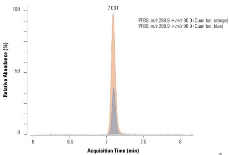
Agilent Ultivo LC/TQ provides robust and accurate measurement of perfluorobutane sulfonate at sub-ppb levels (0.5 ppb).
