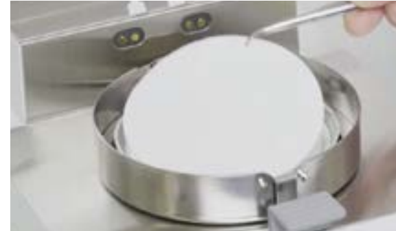
Glass Fiber Filters For liquid and pasty samples
